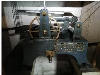
This second mechanism is for the Cambridge chimes which were added in 1917 and is only connected to the clock proper via a single line.
